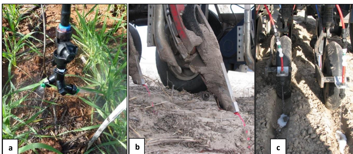
Figure 4. Inter-row droppers used to target fungicide application at the base of wheat tillers to improve in-crop control of crown rot (a); liquid application system used to apply fungicide above (b) and below the seed (c) at sowing to manage Rhizoctonia root rot (photos: Jack Desbiolles, Uni SA)
