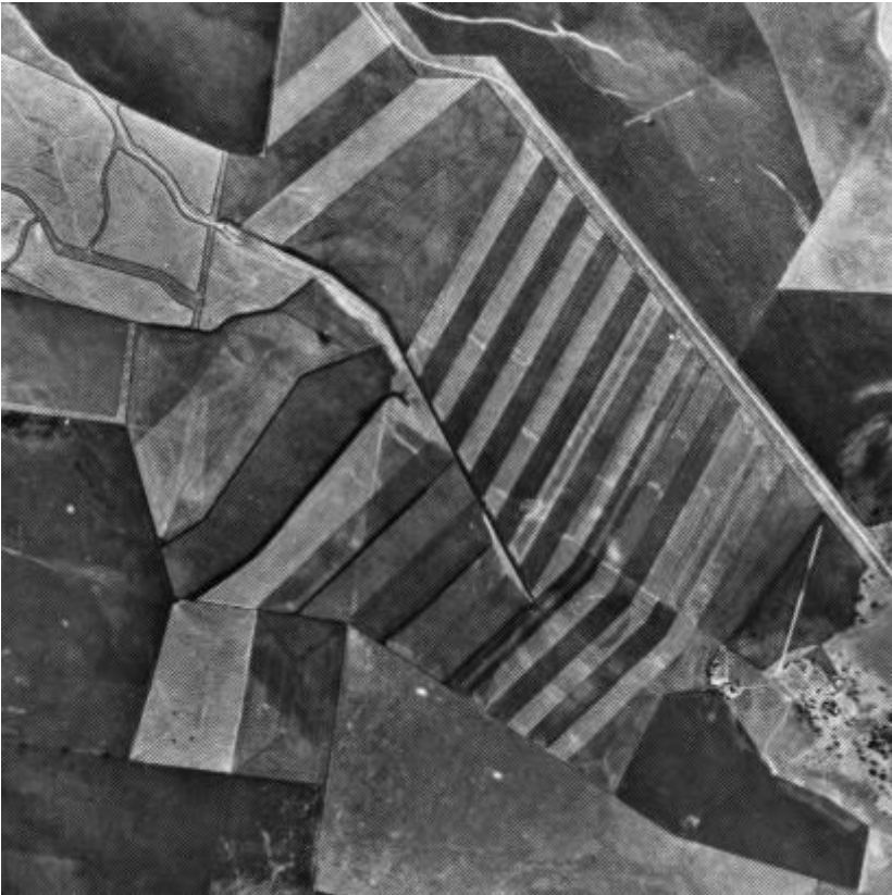
Figure 8.2 The layout of a strip cropping system at Quirindi, New South Wales. The dark strips represent strips prepared for wheat, the light strips are sorghum stubble. The narrow dark lines represent erosion control earthworks. (Photograph reproduced by permission of Soil Conservation Service of New South Wales)
