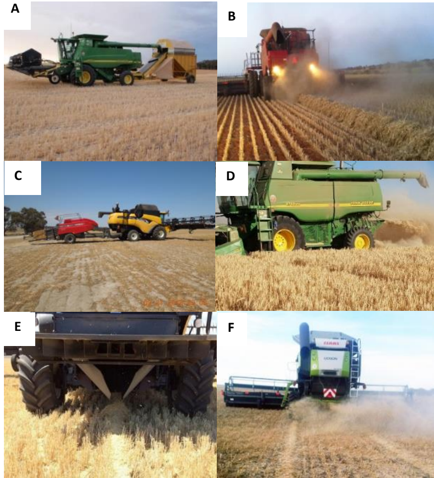
Figure 5. Current forms of harvest weed seed control (A) chaff cart, (B) narrow windrow burning, (C) bale direct system, (D) impact mill, (E) chaff lining and (F) chaff tramlining
