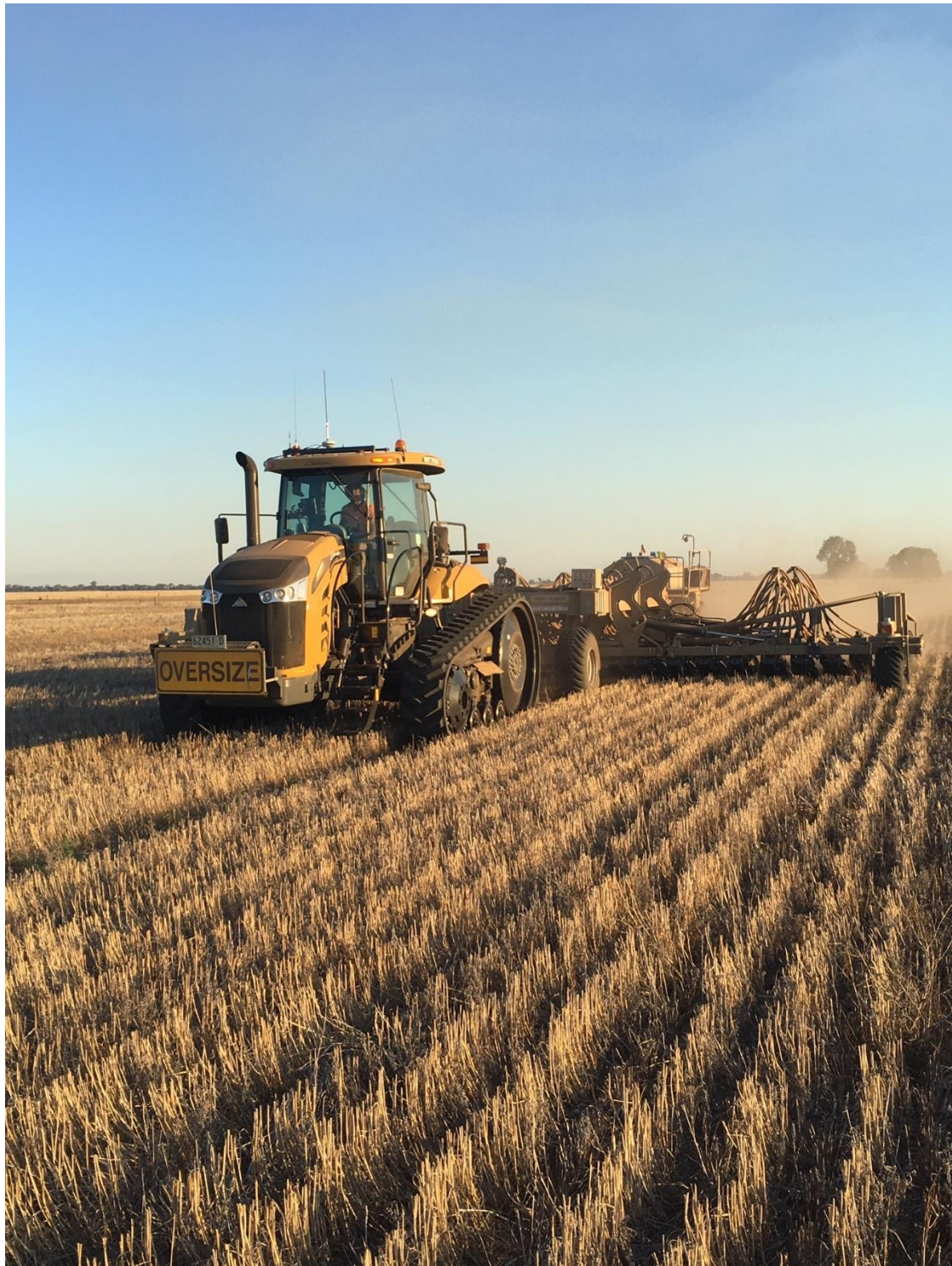
Zero-till disc seeder on 250 mm row spacing, 12 m CTF system, inter-row seeding faba beans using 2 cm GPS guidance into standing barley stubble. (Courtesy: Greg Condon and Stephen & Michelle Hatty, Matong NSW)
