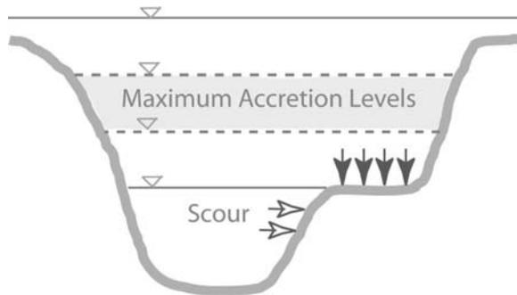
**Figure 6. Conceptual model proposed whereby benches are maintained by flows between benchfull elevation and bankfull, particularly in the range considerably greater than benchfull. Scour can occur due to constant flows lower than benchfull**
