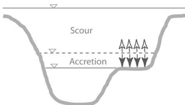
**Figure 1. Conceptual model of current understanding of bench accretion and scour. The dashed line represents the water level at the threshold between accretion and scour.**
