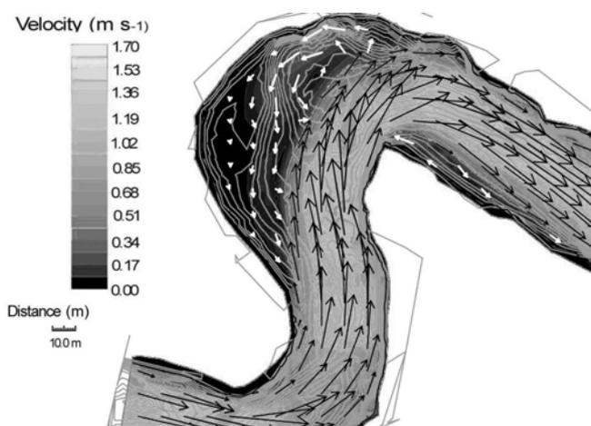
**Figure 5 . Velocity magnitude (shading) and vectors over the site 'Big Eddy' bench (located in the expansion zone top left of channel) at a near-bankfull flow of 157 m<sup>3</sup>/s**
