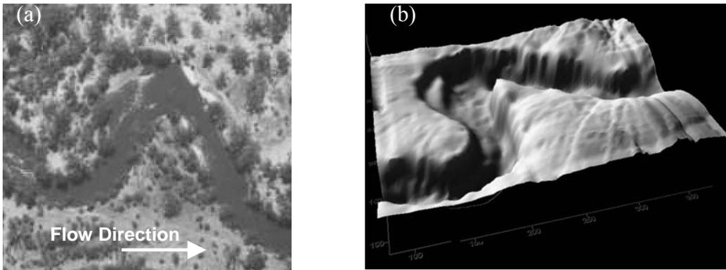
**Figure 3. (a) Site ‘Big Eddy’ bench (top left of bend), Ovens River from 1989 aerial photograph, and (b) three-dimensional representation of this site from survey (plotted in Surfer®), flow left to right**
