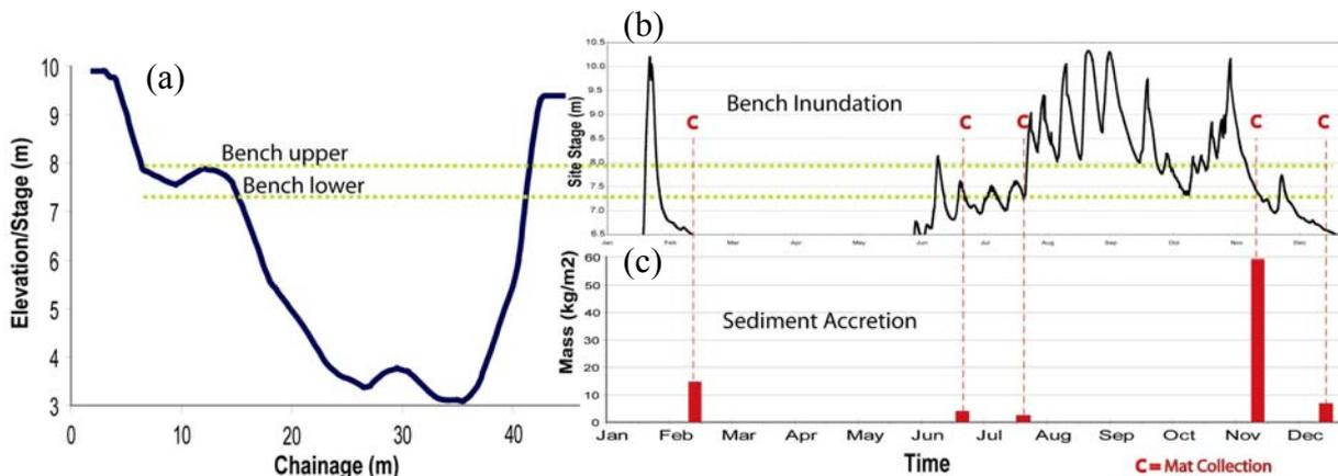
**Figure 4. (a) Cross section of the site ‘Big Eddy’ bench on the Ovens River (note vertical exaggeration), (b) the site hydrograph for the study period of 2005 (relative to bench elevation) and (c) sediment mass deposited from each intervening period**
