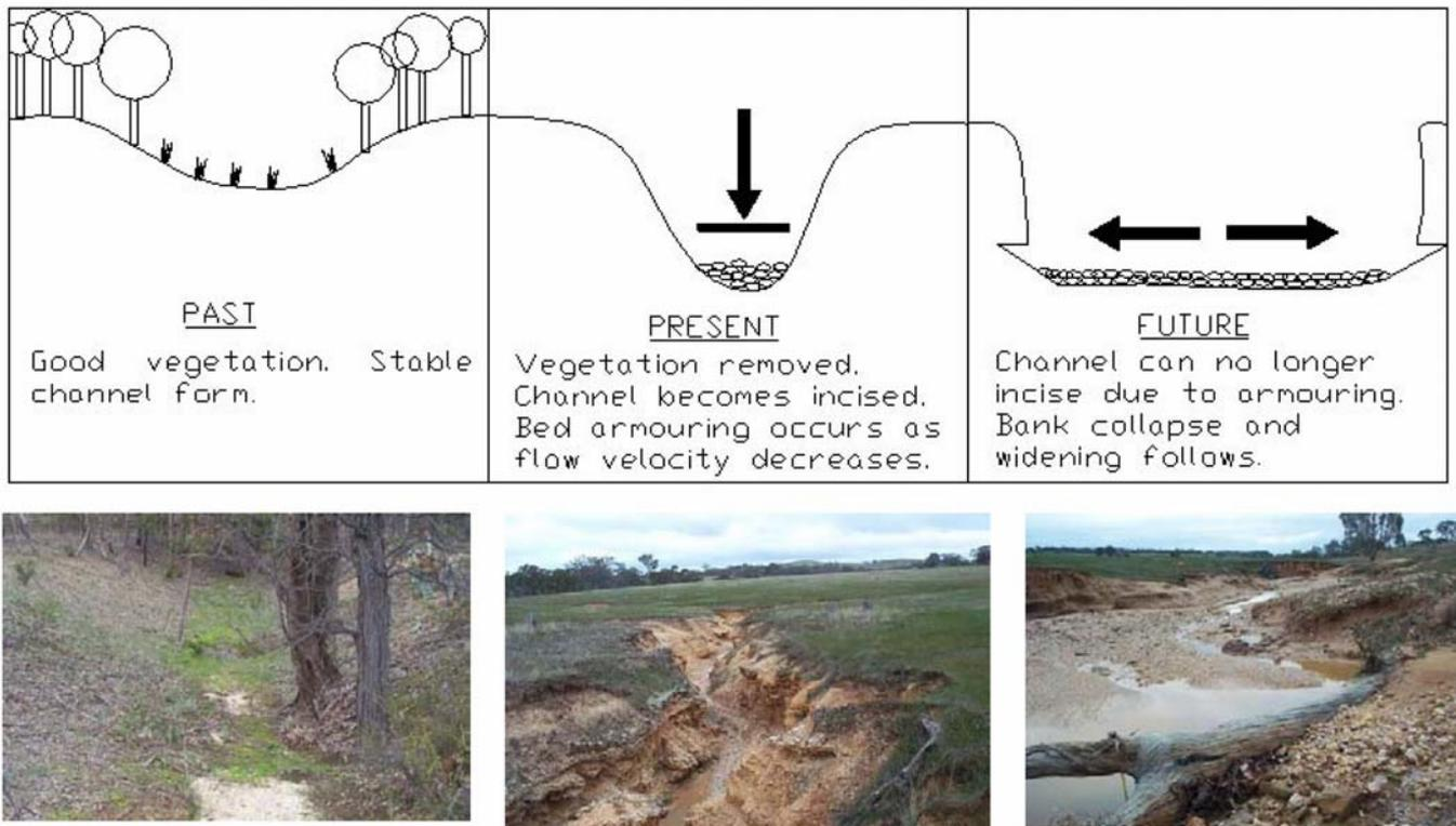
**Figure 2. The process of vegetation removal that leads to stream incision and later bed armoring.**
