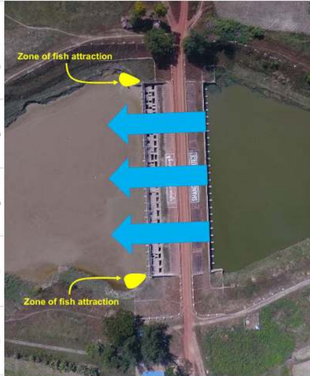
Figure 10. Predicted zones of fish attraction at high flows with uniform flow through all sluice gates.
