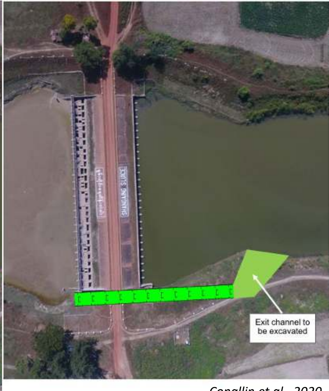
Figure 21. Potential layout of a vertical-slot fishway as a straight channel for construction simplicity.
