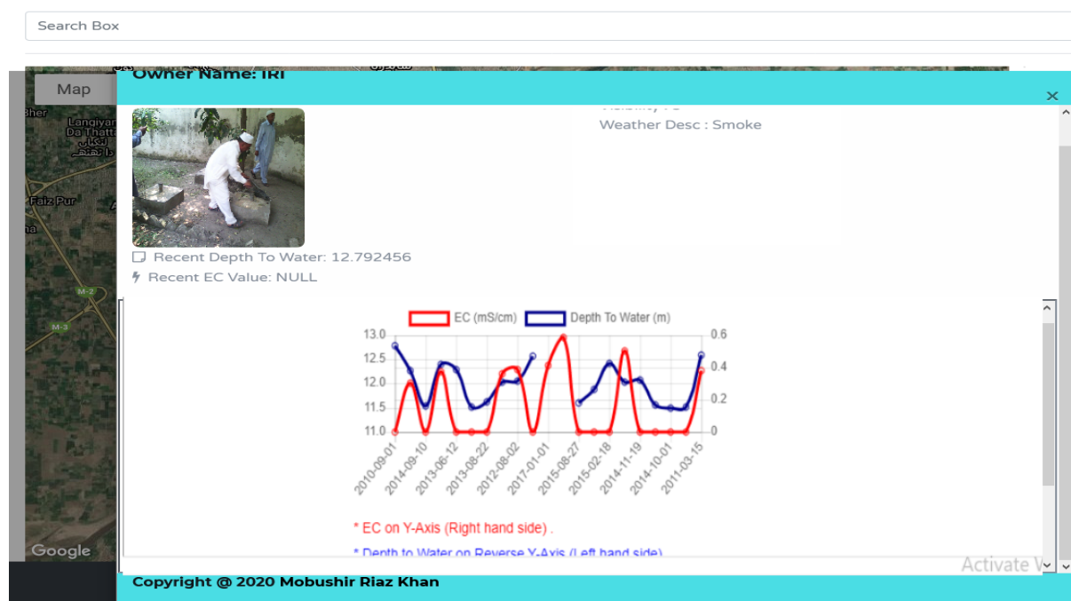
Figure 8: Well information (located at the Irrigation Research Institute Lahore, Punjab)
