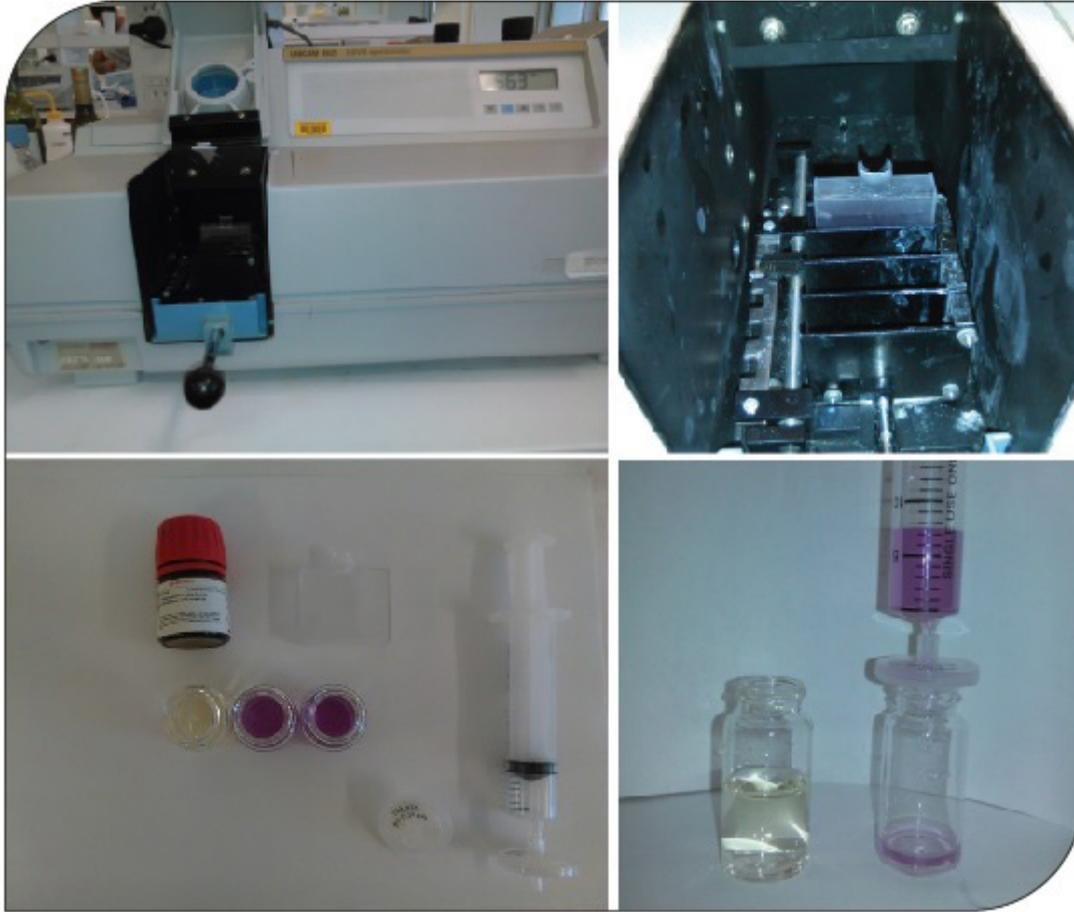
**Figure 2.** Typical spectrophotometer used for the analysis (top left), 40mm cuvette within the spectrophotometer (top right), BCA reagent, sample solutions, including the clear/yellow coloured blank sample, and syringe filter (bottom left), filtration of the samples after the 30 minute reaction time (bottom right).
