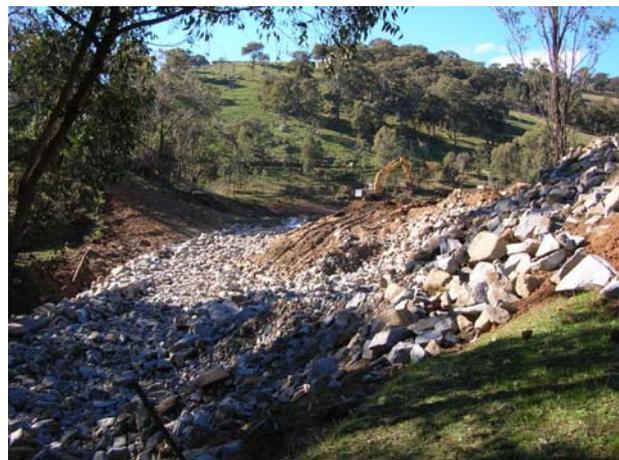
**Figure 4. Embankment with initial breach in place**
