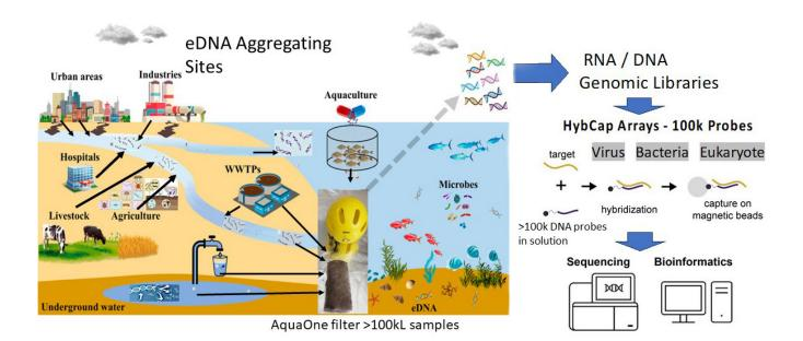
Above: Environmental DNA is collected from natural aggregation sites using nylon filter pads (photo inset shows 24 hours of filtered river water), amplified with droplet PCR, and screened with HybCap Arrays to isolate viral, bacterial, animal and plant targets. (Image, Alan Cooper).
