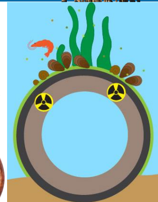
Figure 1. Hypothetical cross-section of an intact pipeline containing NORM-contaminated scale and examples of marine organisms that may be affected. The green layer represents benthic microalgae.
