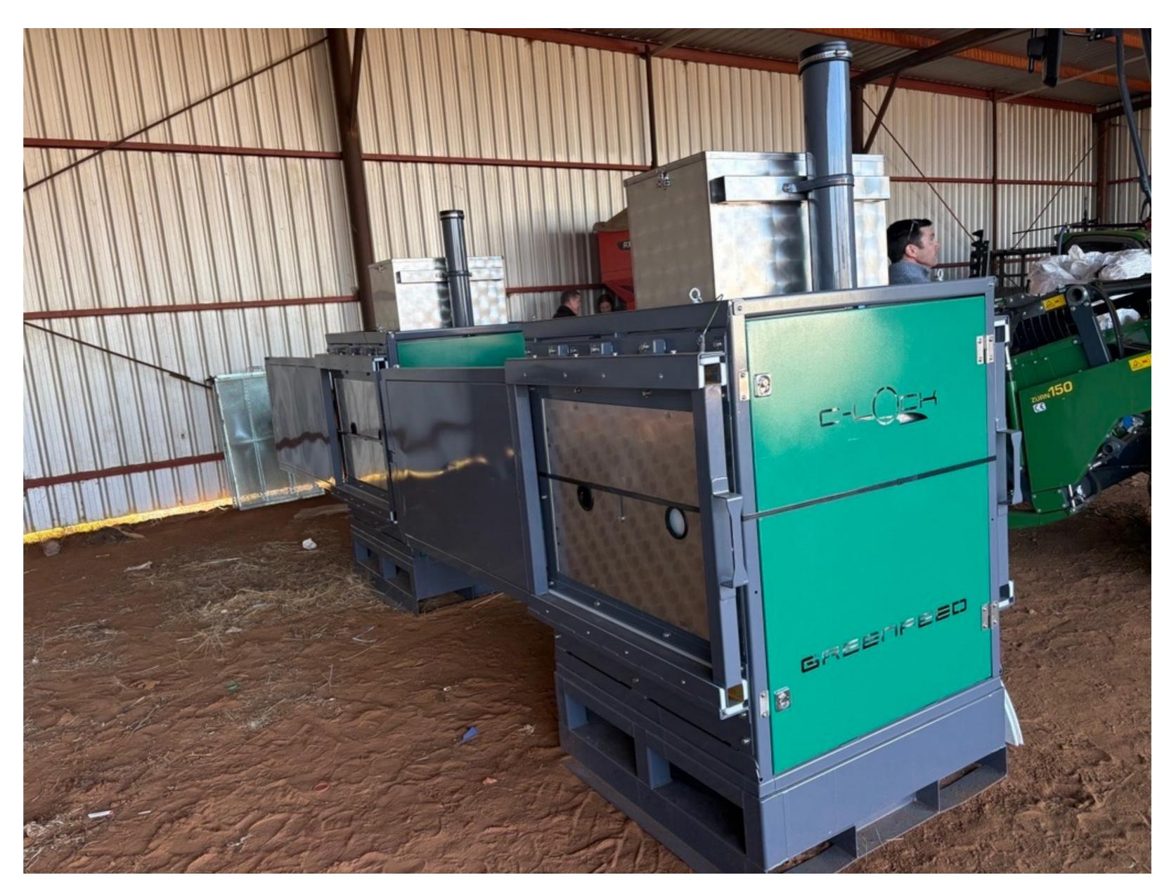
The new unmanned barrow and a C-Lock GreenFeed methan sensor
