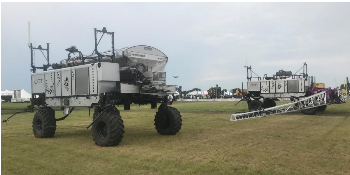
The DOT autonomous platform driving a fertilizer spreader (left) and boom spray (right) on display at Ag-in-Motion field day in Saskatoon Canada July 2019. (Courtesy: John Kirkegaard)
