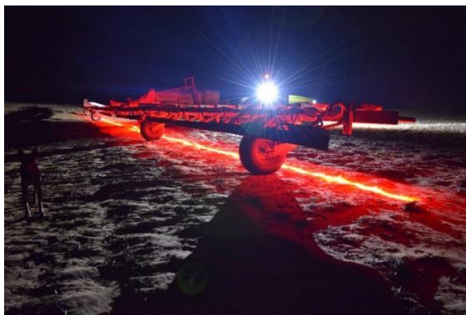
Figure 12. WEEDit sensing light footprint under sprayer boom during night spraying of summer weeds (picture courtesy of Bulla Burra farm)
