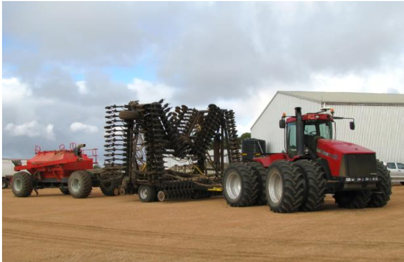
Figure 4. Large scale air seeder CA equipment for broadacre crops are commonly 12-24 m wide, set at 220-300 mm seed row spacing and can sustain effective work rates in the range of 15-25 ha/hr (picture by Jack Desbiolles)
