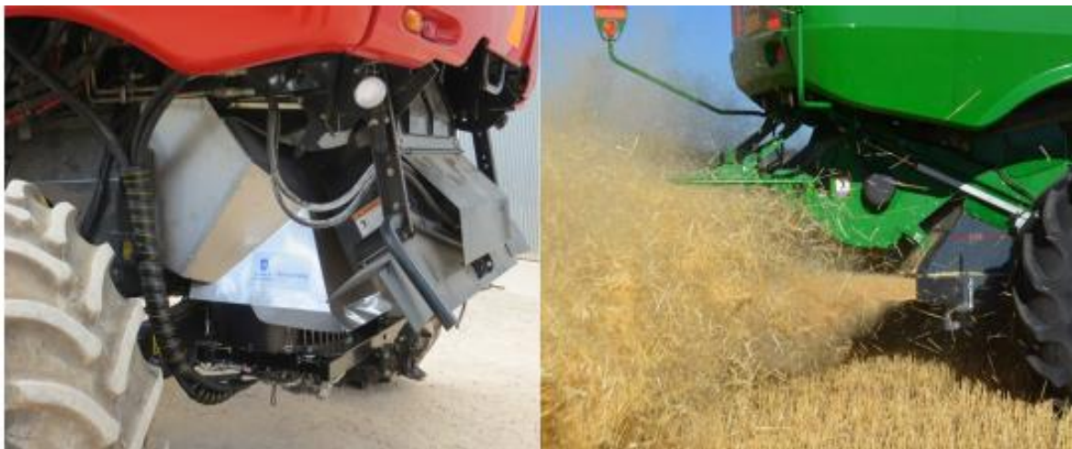
Figure 15. Weed seed destruction at harvest is a recent Australian innovation that is a game changer for sustainable weed management in CA systems . Left: close-up view of iHSD early prototype with hydraulic drive (picture by Chris Saunders) Right: Seed Terminator unit in operation below a conventional straw chopper (picture courtesy of Seed Terminator)
