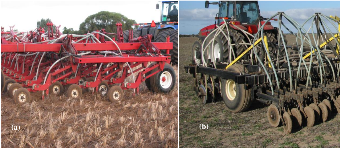
Figure 5. (a) A majority of CA seeders in Australia use tyne seeding systems, (b) Recent interest in disc seeding systems is especially increasing among long term CA farmers (pictures from Jack Desbiolles)
