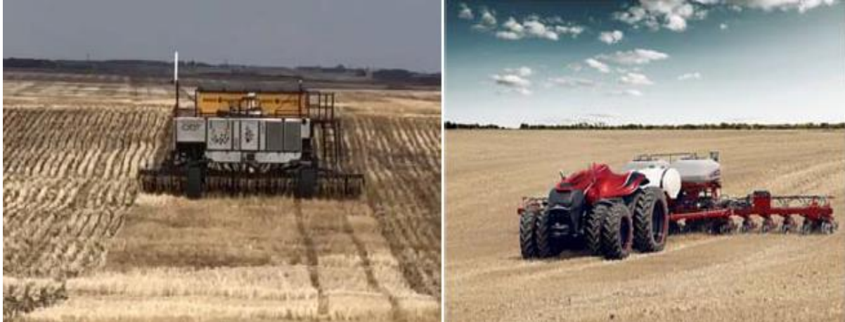
Figure 3. Left: DOT autonomous tractor and no-till seeder tested in Canada since 2017; Right: CNH industrial autonomous tractor concept (pictures courtesy of Norbert Beaujot, SeedMaster, and CNH respectively)
