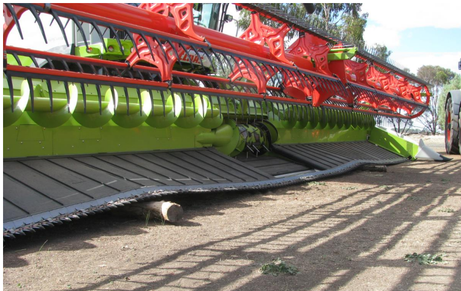
Figure 13. Flexi-belt fronts can follow ground contours across their width with a 225 mm flex range (e.g. Claas Convio Flex front, picture by Jack Desbiolles)
