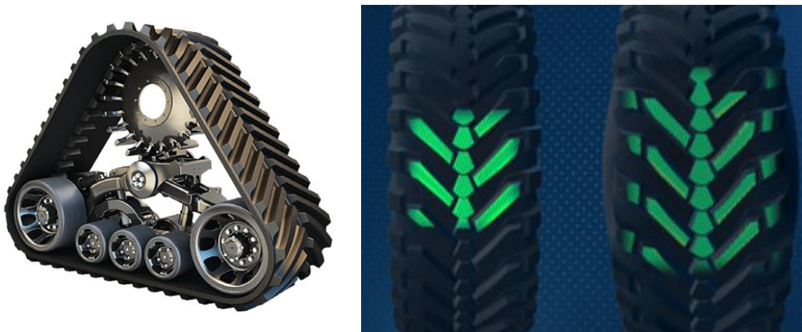
Figure 2. Left: Track suspension technology improving the riding stability in rough terrain ( e.g. ATI Inc. Power-Flex Trax™ with Terraform™ suspension), Right: New adaptive tyre technology ( e.g. Michelin EvoBib) maximising footprint under field setting (0.4 bar) vs optimum road footprint at 1.8 bar via the use of a central tyre inflation system (pictures courtesy ATI and Michelin, respectively)
