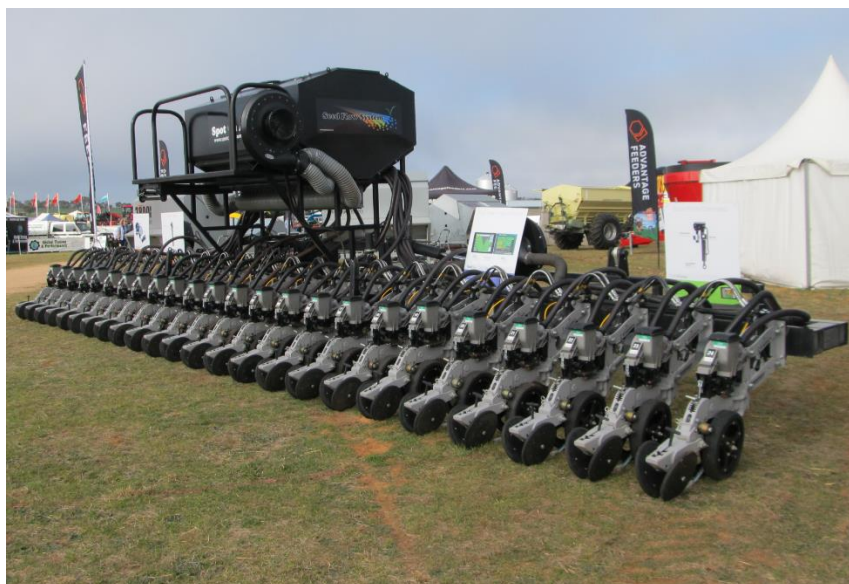
Figure 8. Precision planting technology adapted for winter grain crop sowing is the new frontier of CA mechanisation in Australia (picture from Jack Desbiolles)
