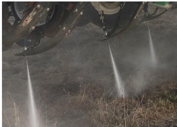
Figure 7. Recent research showed the Aqua-Till™ waterjet cutting capacity of wheat residue is proportional to the nozzle orifice area, and exceeds 35 t/ha with a 0.3 mm nozzle size (picture from Greg Butler)
