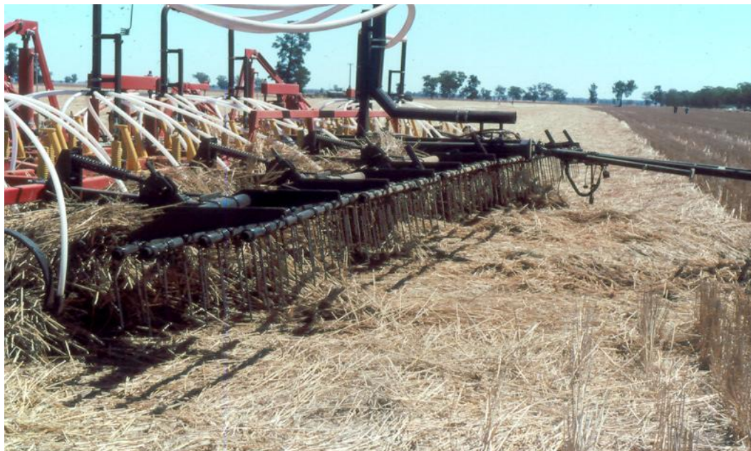
Challenges: Stubble trouble with high residue load (around 7 t/ha), long straw and inadequate machinery clearance (Courtesy: Jim Pratley)
