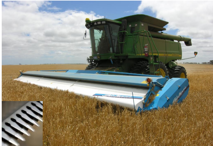
Figure 14. Stripper fronts use multiple rows of stripping fingers (inset) and help maximise the proportion of anchored residue retained in CA systems, e.g. Shelbourne Reynolds (picture by Glen Riethmuller)
