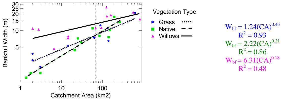
**Figure 1. Scatter plot and regression equations showing the relationship between vegetation type (willows, natives or grass), bankfull width and catchment area (log-log scale). The vertical dashed line indicates the point at which sites with natives become narrower than those with grass (~60km<sup>2</sup>).**
