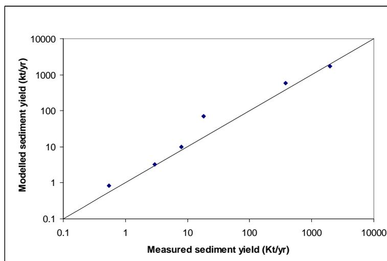
**Figure 2. Measured versus modelled sediment loads for six Burdekin River sub-catchments.**
