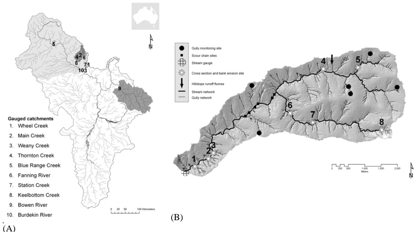
**Figure 1. (A) map of the Burdekin sub-catchments currently monitored for sediment loads and (B) the Weany Creek catchment showing the location of the hillslope, gully and bank erosion measurement sites.**
