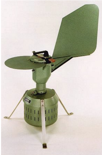
Figure 10.2: Burkard spore trap
