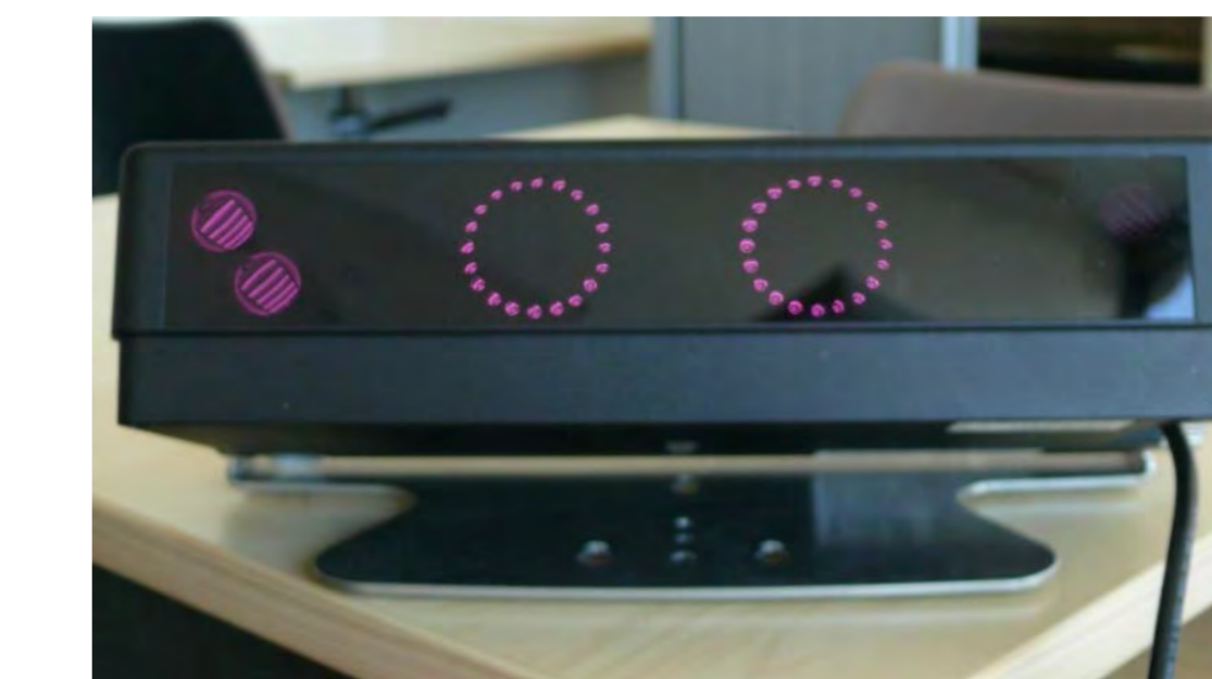
Fig. 5: Tobi X120 eye tracker has been employed in collecting data (picture courtesy: www.wired.com).
